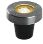
Umbra 3152051 Warm white 3W - 190 lumen - A+ Stainless steel 85 x 105 mm (HxW) Borehole 70 mm Ø
